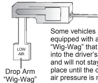
Some vehicles are equipped with a "Wig-Wag" that drops into the driver's view, and will not stay up in place until the desired air pressure is restored.
