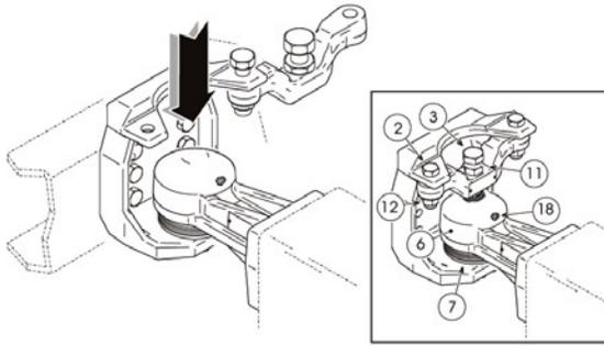
**Step 6. Protect Coupling Ball and Anchor Edge onto Ball**
