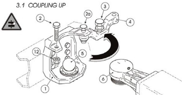
**Step 1. Remove Safety Lock Screw and Rotate Safety Cover Bar**
