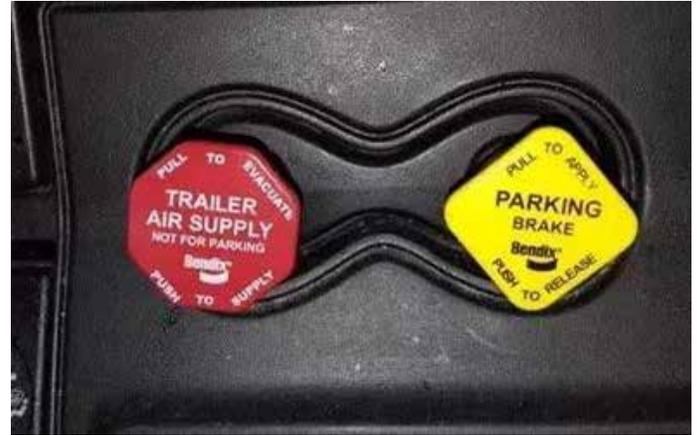
You pull the knob out to evacuate the air from the brake chamber and put the parking brakes (spring brakes) on, and push it in to release them. On older vehicles, the parking brakes may be controlled by a lever. Use the parking brakes whenever you park.
