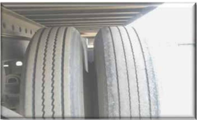
**Figure 11.29 Proper Wheel Spacing**
