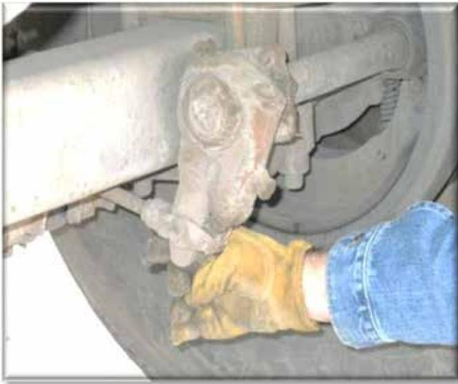
**Figure 11.56 Slack Adjuster and Pushrod**
