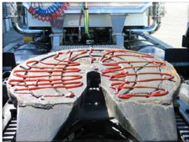
**Check if fifth wheel is in proper position for coupling:**
