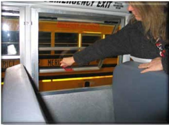
**Figure 11.72 Window Alarm Check**
