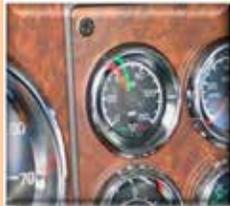
At 20-45 psi, tractor protection valve should pop out.
