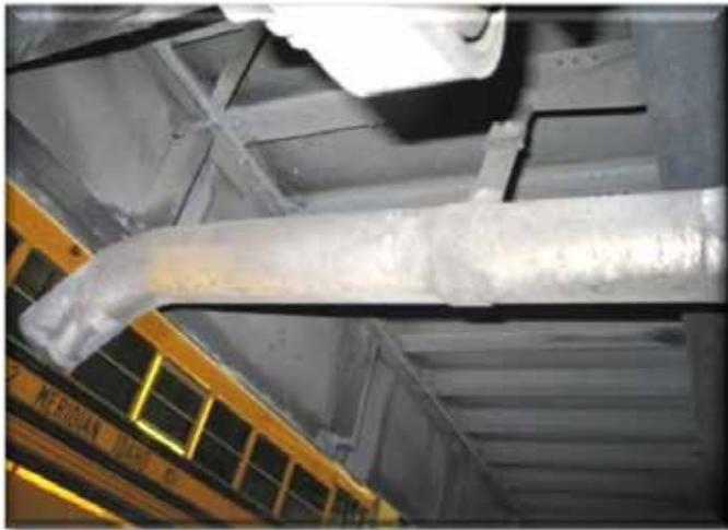
**Figure 11.78 Under Bus Exhaust Pipe Check**
