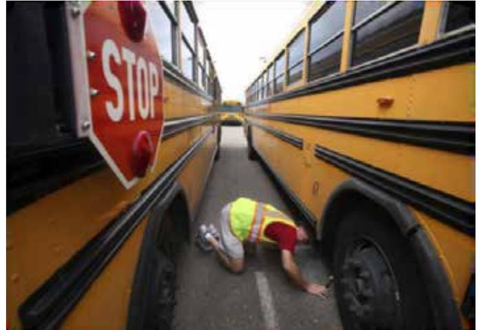
**Figure 11.76 Under Bus Fuel Leak Check**
