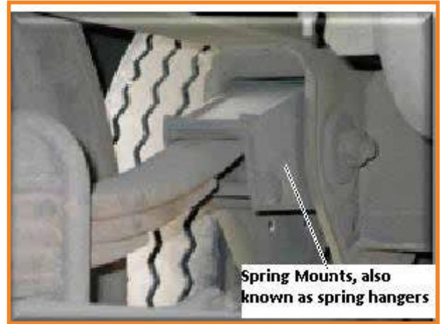
**Figure 11.54 Spring Mounts / Spring Hangers**
