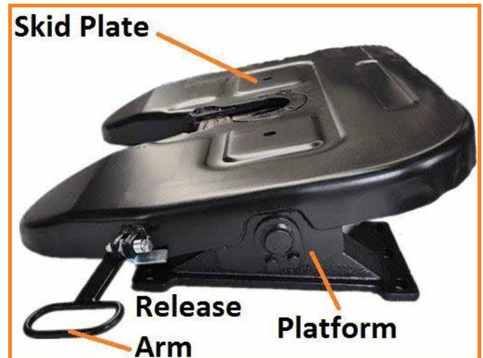
**Figure 11.42 Fifth Wheel Skid Plate Components**
