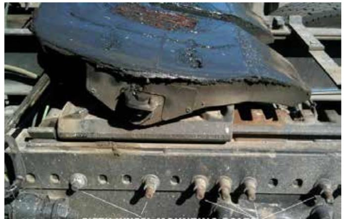
**Figure 11.38** Fifth Wheel Mounting Bolts
