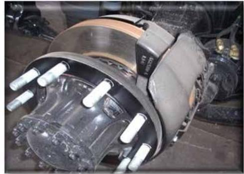
**Figure 11.57 Brake Drum and Brake Rotor**
