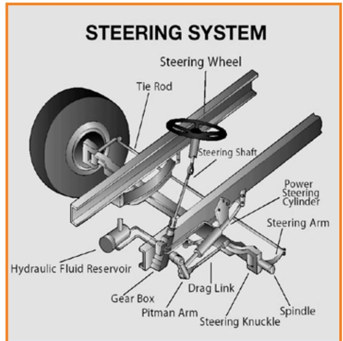
**Figure 2.1 A typical steering system**
