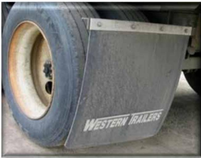
**Figure 11.34 Properly Mounted Mud Flap**
