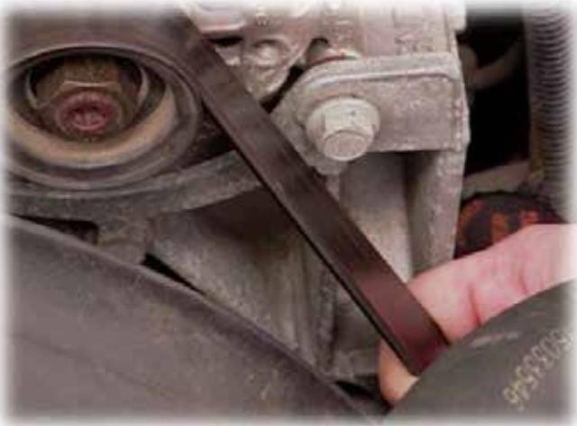
**Figure 11.3 Checking Belt Tension**
