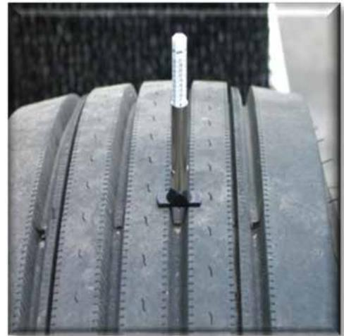
**Figure 11.28 Checking Tire Tread Depth**
