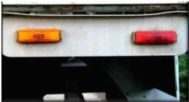
**Figure 6.9 ABS Malfunction Warning Light**
