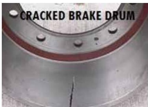
**Figure 11.24 Cracked Brake Drum**
