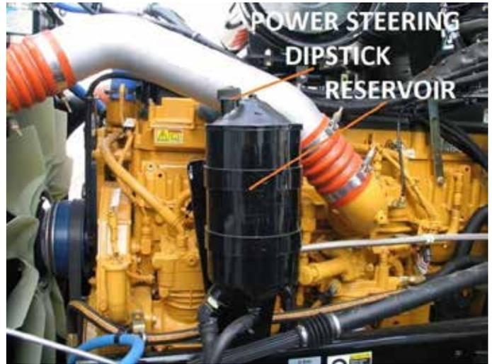
**Figure 11.4 Power Steering Components**
