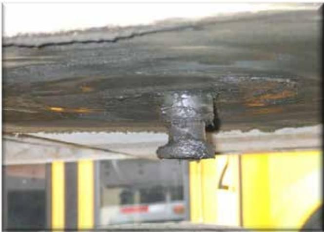
**Figure 11.44 Trailer Kingpin and Kingpin Plate**
