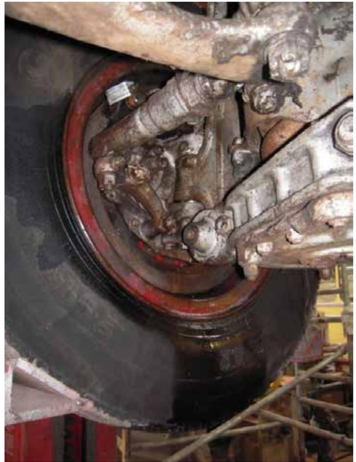
**Figure 11.26 Brake Mounts**
