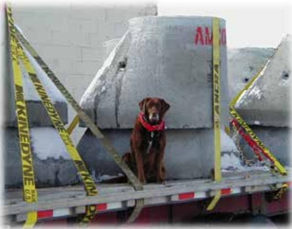
In closed vans, tie-downs can also be important to prevent the from cargo shifting which may affect the handling of the vehicle. Tie-downs must be of the proper type and proper strength.
