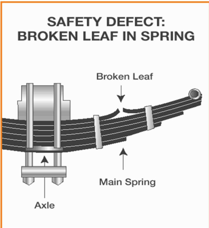
**Figure 2.3 Broken Leaf Spring**
