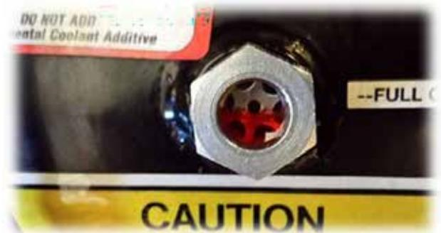
Figure 11.2 Coolant Level Sight Glass
