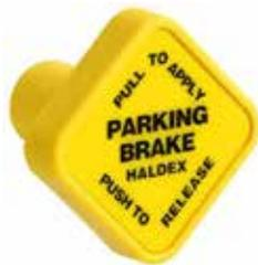
Don't use the parking brakes if the brakes are very hot (from just having come down a steep grade), or if the brakes are very wet in freezing temperatures. If parking brakes are used while the brakes are very hot, they can be damaged by the heat. If they are used in freezing temperatures when the brakes are very wet, they can freeze and the vehicle cannot move. Use wheel chocks on a level surface to hold the vehicle. Let hot brakes cool before
