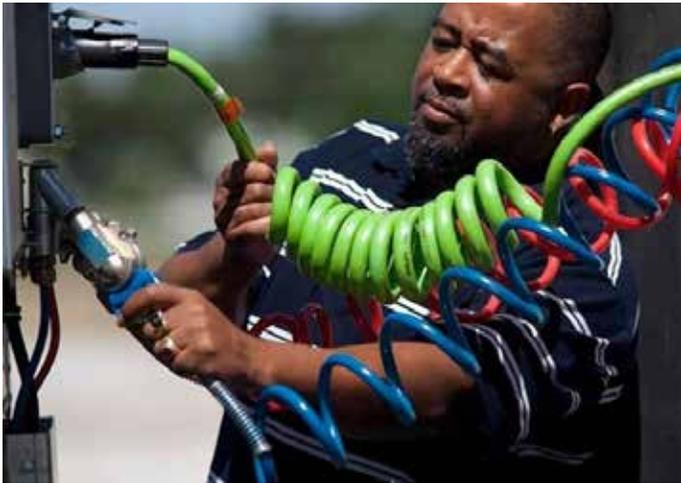
**Figure 11.36** Secure Air and Electric Line Connections
