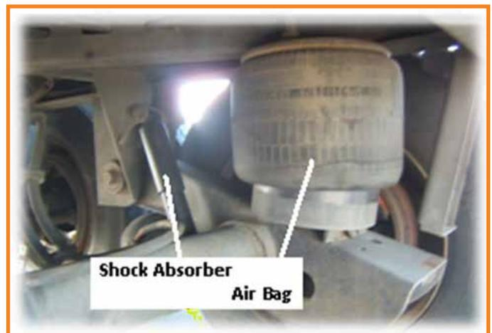
**Figure 11.55 Shock Absorber and Air Bag**
