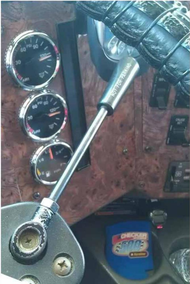
***The trailer hand valve on this International tractor is located on the steering column.***
