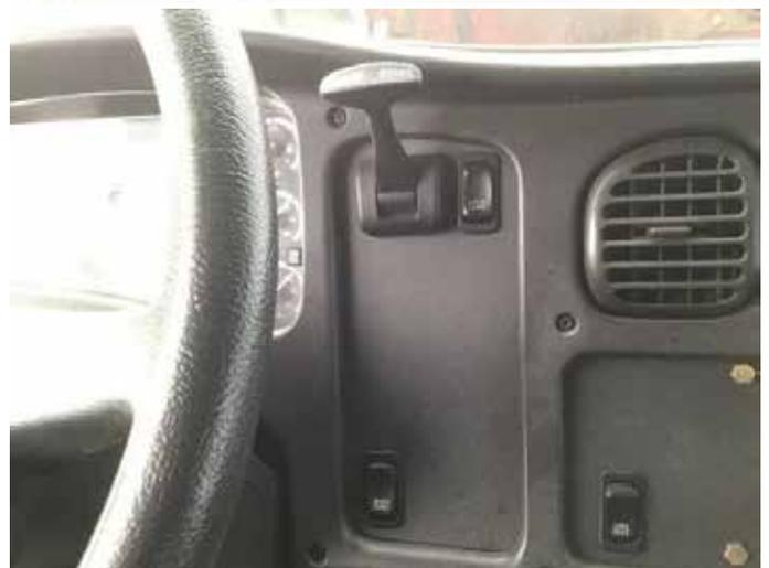
Trailer Brake Handle in Freightliner Tractor
