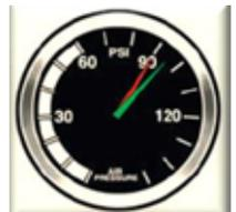
system, or a single gauge with two needles. Dual systems will be discussed later. These gauges tell you how much pressure is in the air tanks.
